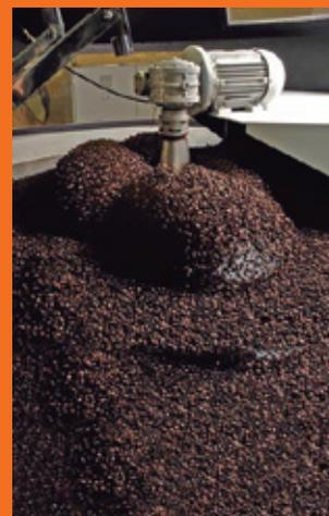
The Opus 4<sup>th</sup>. Generation, is possible to draw the coffee temperature curve and the roaster will do the setting of the air flow, temperature, pressure and drum rotation in order to reach that coffee temperature throughout the roasting process.
